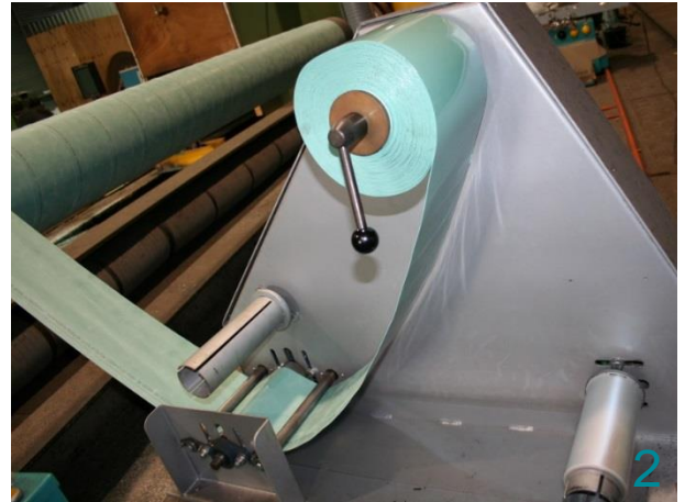
2 Depending on pipeline diameter, the angle of the FAST Basecoat Wrapping Device must be adjusted to ensure a minimum 10mm side-by-side overlap.
