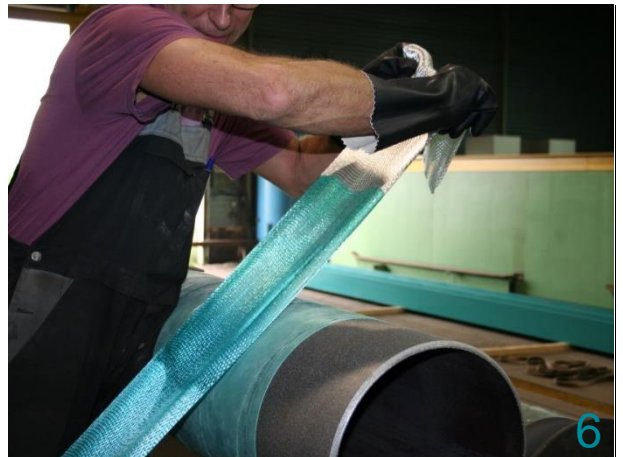
6 Pull the impregnated GAST GRE Fabric through the GRE Wrapping Device and place it on the FAST Basecoat GRE.
